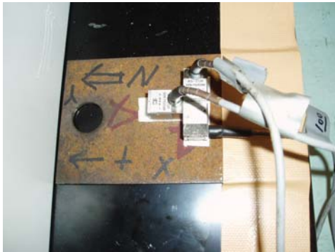
Acceleration on server rack Photo 3-1
